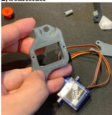
install 9g servo on gearholder. Servo come with self tapping screw. Usethis screw and assemble.
