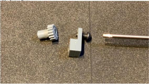
With M3\*6Bottun screw the shaft must spin easily.
