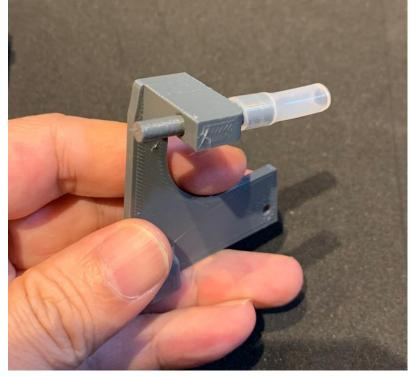
And then insert the shaft. If the hole is tight, smoothing the hole using a 4 mm drill
