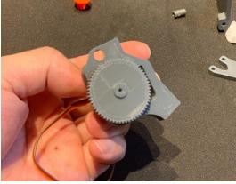
And set the gear with self tapping screws that come with the servo.
