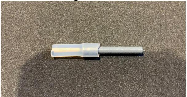
Cut the silicon tube 22mmand connect the steering shaft.
