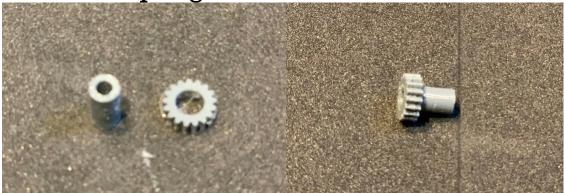
Check output 17T gear and shaft. Gear should apply for hole side. When assembling them, apply
