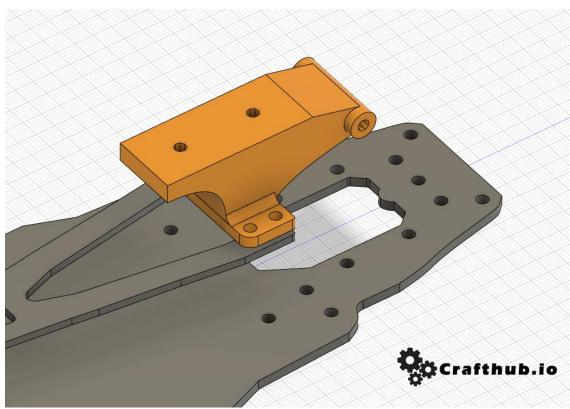
Remove M6\*23mm post and install Battery mount Base
