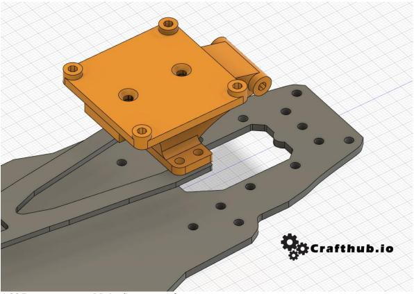
Add Battery mount M3\*6 Countersunk screw
