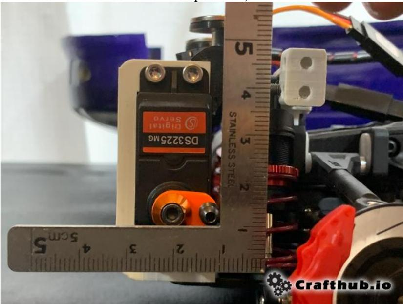
Servohorn and endball fix with M3x8 cap screw
