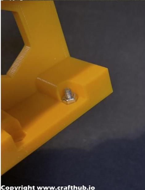
Use the screw to pull the nut into M3 Nut position
