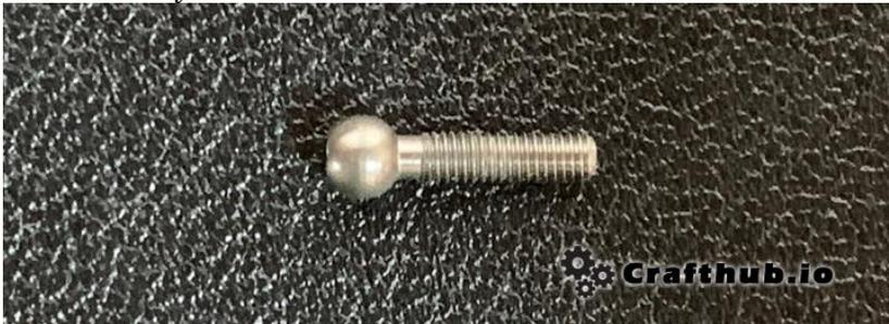
Assemble the front Strut tower by adding M3\*15 screws for the front. Do not over tighten. Check
