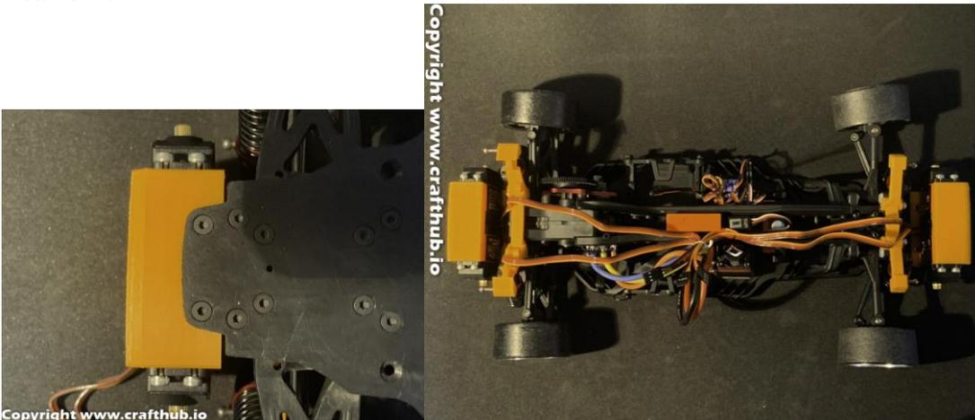
Remove the original bumper and replace to Servo holder.
